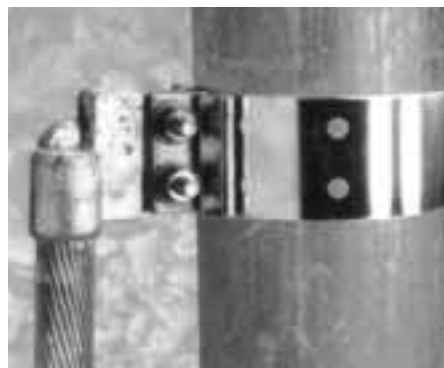
Figure 9. ERITECH Pipe clamp fitted to metal pipe with conductor stub CADWELD exothermically welded to copper conductor.
